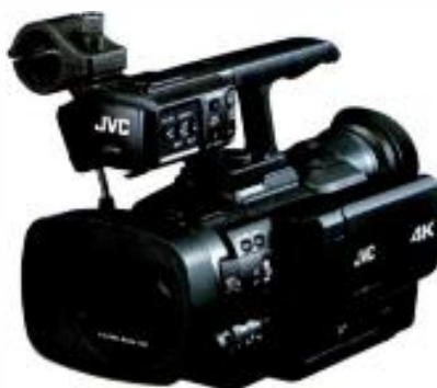
The JVC GY-HMQ10 combines a 1/2in CMOS imager with 8.3 million active pixels and a Falconbrid LSI processor to record, and play 4K video in real time at 24p, 50p or 60p.
